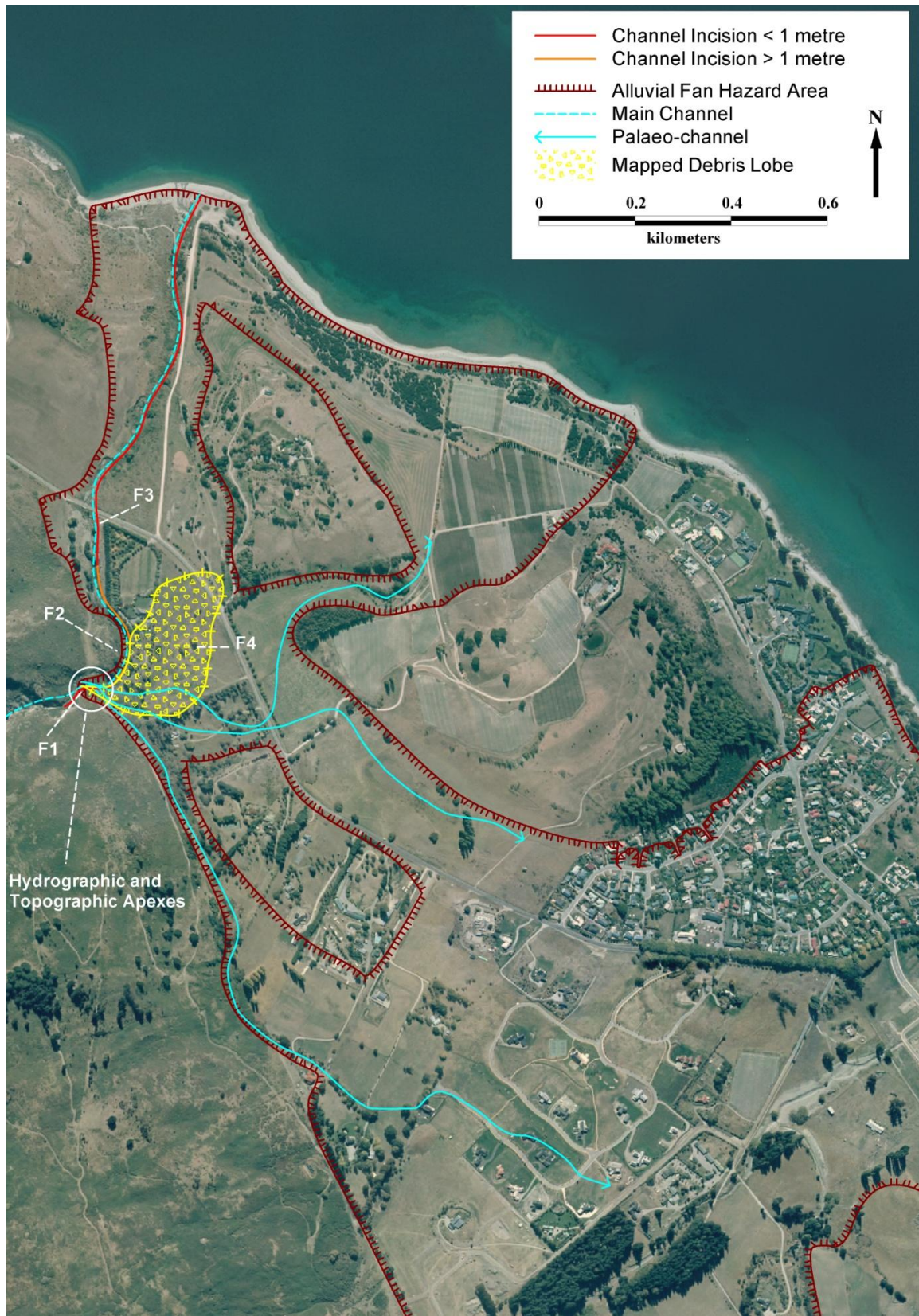
Figure 6.5 Waterfall Creek alluvial fan, noting some key alluvial-fan features; aerial photo taken in March 2006
