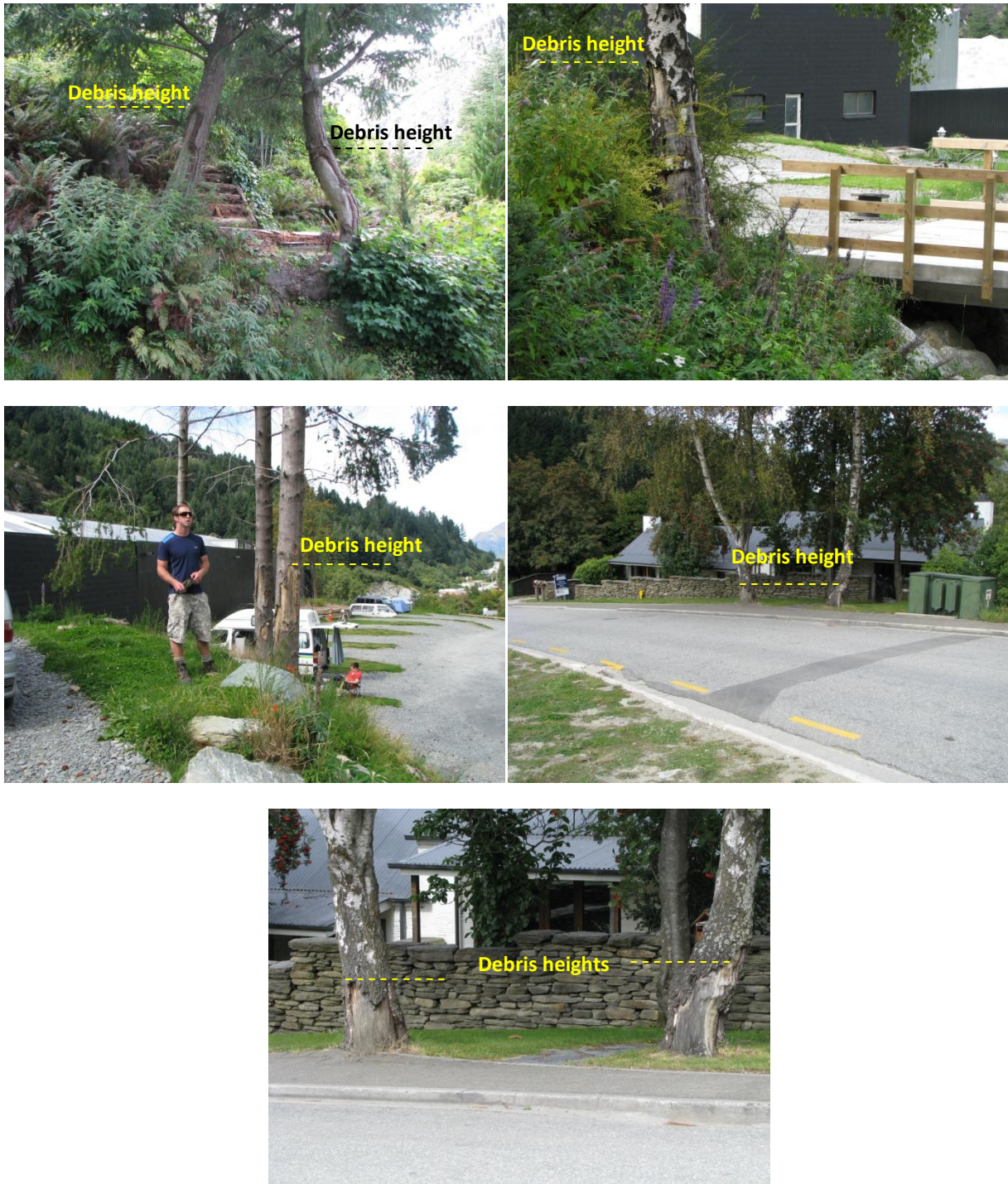
Figure 10.7 Debris-impact scars on mature trees on the Brewery Creek alluvial fan. Top left: Debris scars on left-bank trees just upstream of point 005 (Figure 10.4). Top right: Debris scar on true-left tree at point 005. Mid-left: Debris scars on trees at point 006 with figure for scale. Mid-right: Looking across Bowen Street towards trees at point 008. Lower image: Trees on far side of Bowen Street at 008
