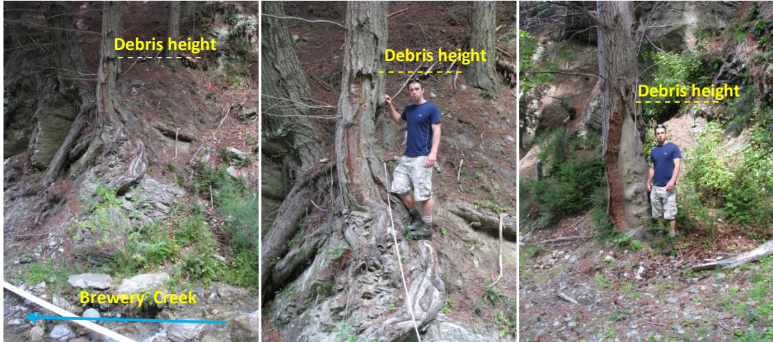
Figure 10.6 Debris-impact scars on mature trees near Brewery Creek’s topographic apex. Left: Debris mark at 003 (Figure 10.4), showing height with respect to ground level. Centre: Same tree as left image, with figure for scale. Right: Similar tree just downstream of mark 003
