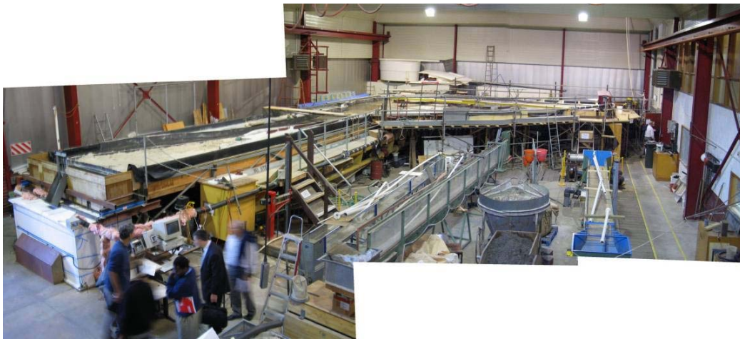
Figure 6.1: Physical model of Shotover River delta
