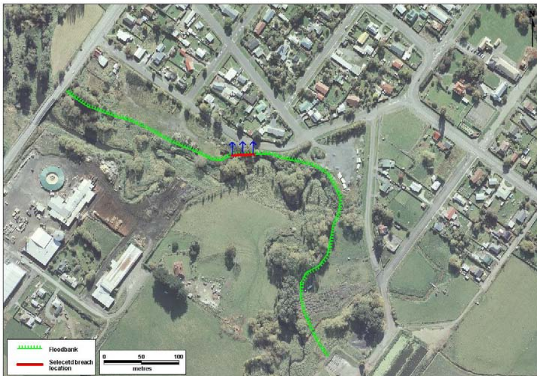
Figure 12. Floodbank breach location for the selected breach scenario.
