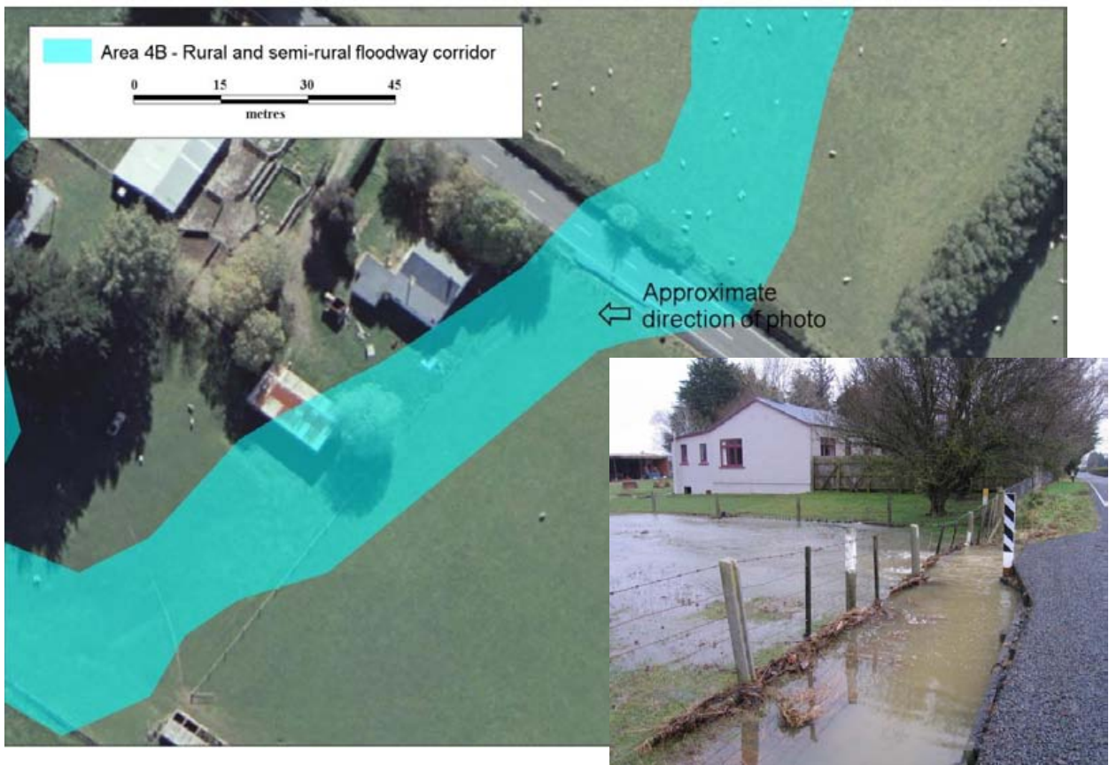
Figure 10. Example of a floodway crossing Springfield Road. The location and direction of the photo (inset) taken during a rainfall event in July 2008 is also marked on the image. The photo does not show floodwater covering the full extent of the floodway corridor, although the July 2008 event was a reasonably small magnitude event (an analysis using flow record from 1981 to 2012 at the Tokomairiro at the west branch bBridge site shows this event was slightly larger than an annual flood).
