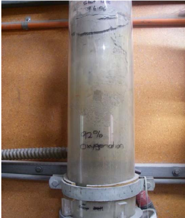
Figure 1: Example kinetic leach test column.
