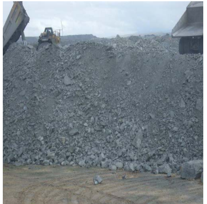
Plate 8. Rock Stack showing segregation of waste with coarse rock at base of lift
