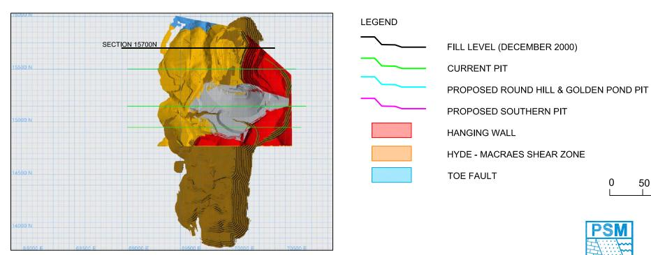
FOOTWALL FAULT & HANGING WALL SECTION 15700N
