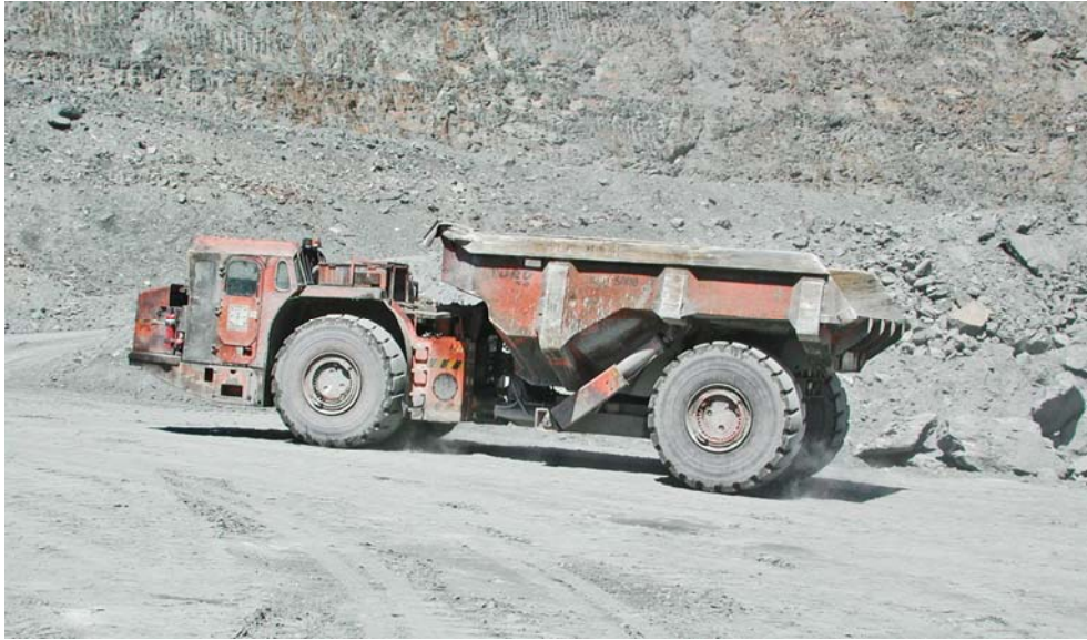
Figure 9. Underground Dump Truck
