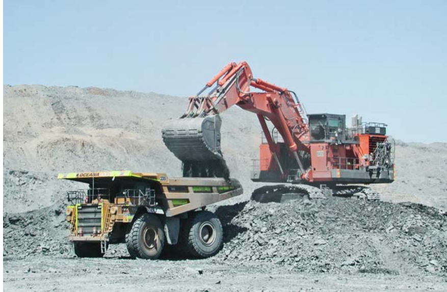
Figure 5. HitachiEX3600 Excavator Loading a Cat 789C Dump Truck
