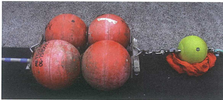
Figure 2.1 The S4 current meter (right) and the 160 kg buoyancy set.
