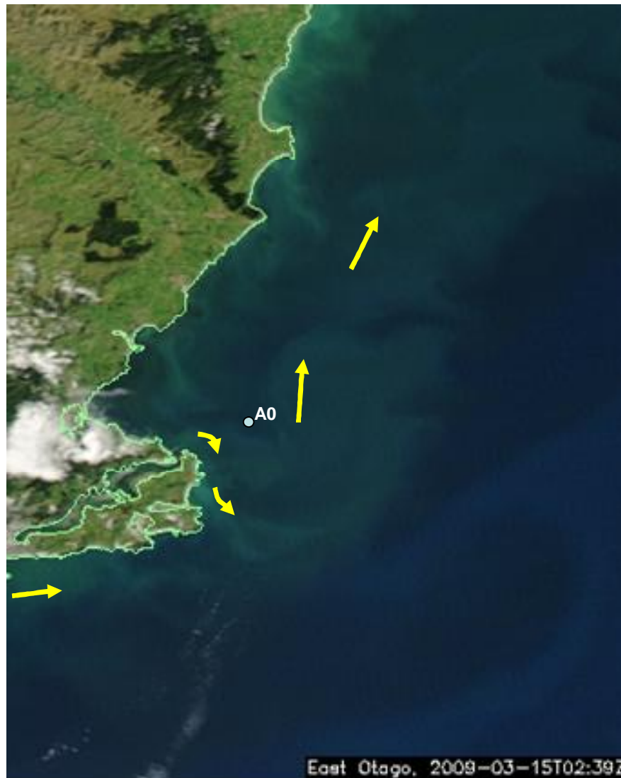
Figure 6: Example of a pan-sharpened 250-m resolution MODIS satellite image taken at 1439 (NZST) on 15 March 2009. A light north-east wind was present during the previous 24 hours preceded by 36 hours of south-west winds. The superimposed arrows highlight the circulation patterns approximately inferred from the naturally-occurring plumes, including the north to north-east drifting plumes offshore in the main Southland Current beyond A0. [Source: NASA and processed by NIWA]
