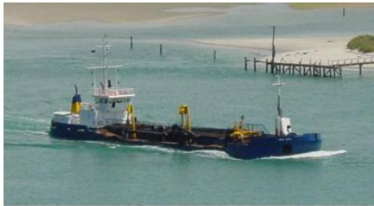
Figure 1 – Port Otago Trailer Suction Dredge "New Era"
