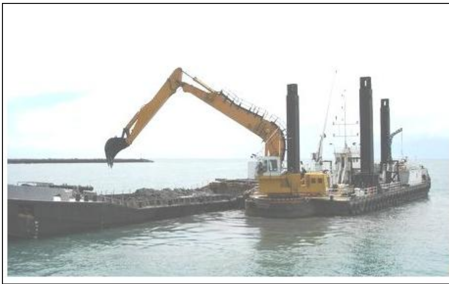
Figure 3 –Backhoe Dredge Machiavelli (Heron Construction Ltd)
