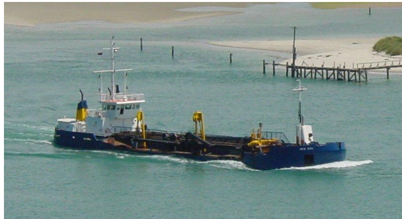
Figure 5.1 Port Otago Ltd Trailing Suction Hopper Dredge New Era
