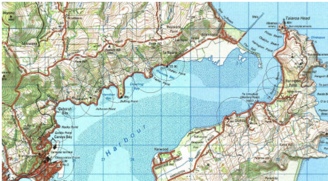
Fig. 10 Zones inside which a dredge of 110 dB L w would exceed 45 dB A at a dwelling (590 metre radius from dwelling)
