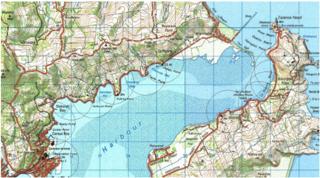
Fig. 9 Zones inside which a dredge of 112 dB L w would exceed 45 dB A at dwelling (750 metre radius from dwelling)
