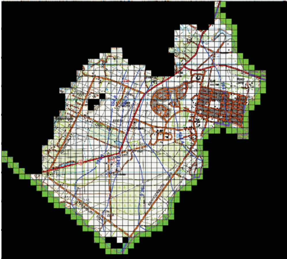
Figure 9: Numerical model boundaries: river (RIV) in green, head no flow (HNF) in black.
