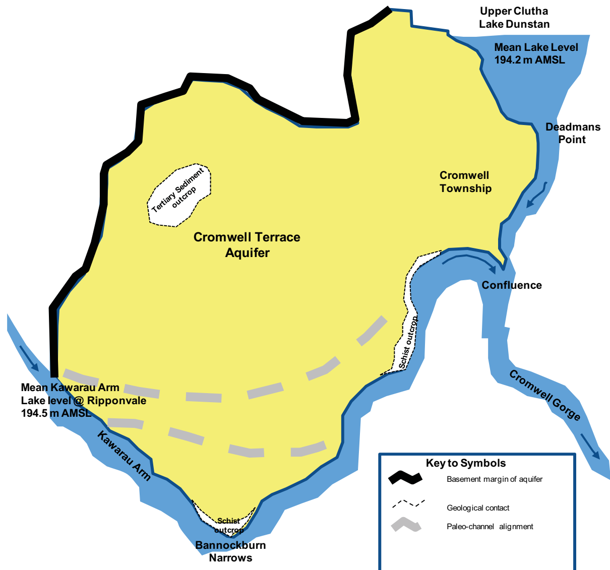
Figure 7: Conceptual outline map of the Cromwell Terrace Aquifer, showing extent in yellow, paleo-channel alignments in gray and approximate post-filling lake levels.
