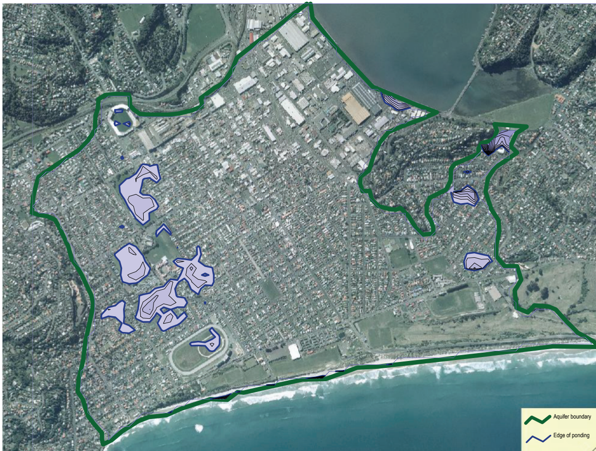
Figure 5: Above ground ponding of groundwater for Scenario 3 considering 0.4 m of sea level rise.
