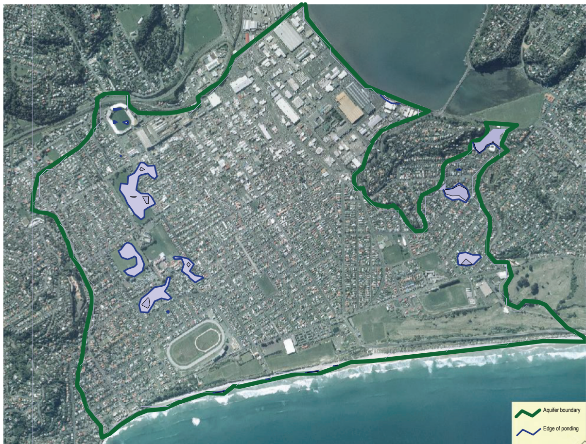
Figure 2: Above ground ponding of groundwater for Scenario 0 considering nil sea level rise.
