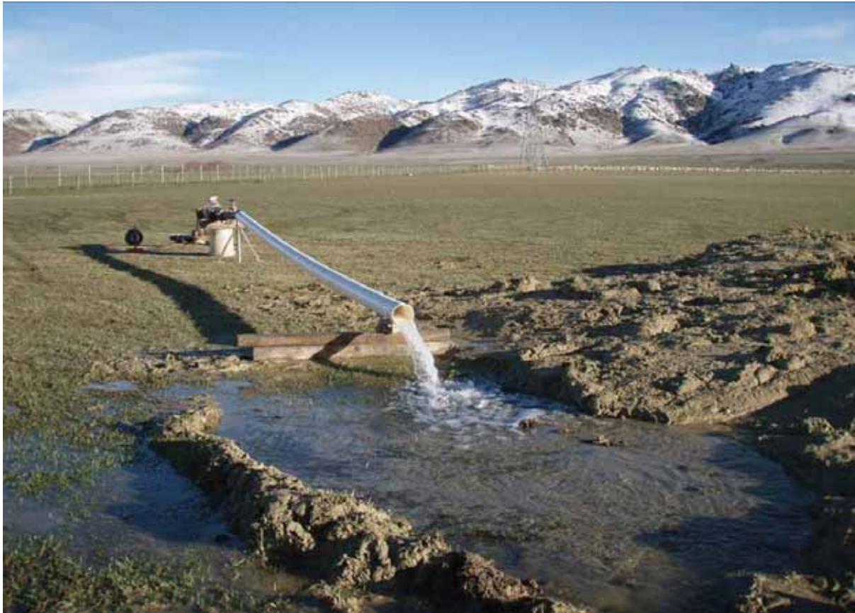
Figure 11. The 24-hour constant rate pumping test carried out on the Meade Road bore.
