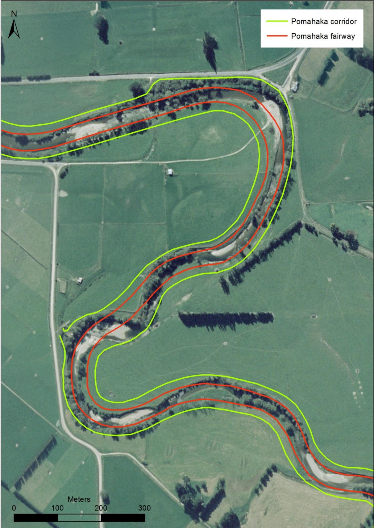
Figure 18. Pomahaka River mapped fairway deviating from the current channel alignment (aerial photography collected in 2006)
