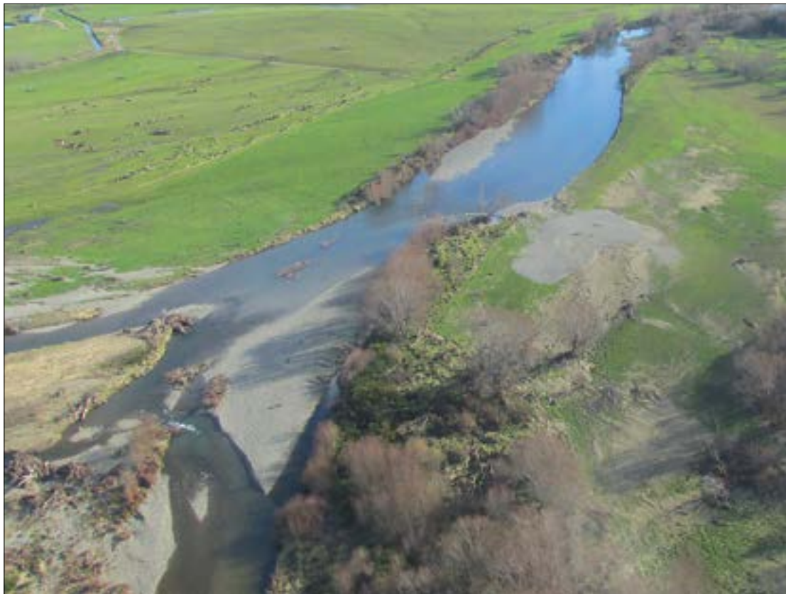
Figure 2. Examples of recent changes in channel morphology. Top: Bank erosion on the true-right bank of the Kauru River (June 2013). Bottom: Bank erosion and sediment deposition in the Kākaunui River downstream of Gemmells Crossing (May 2014).
