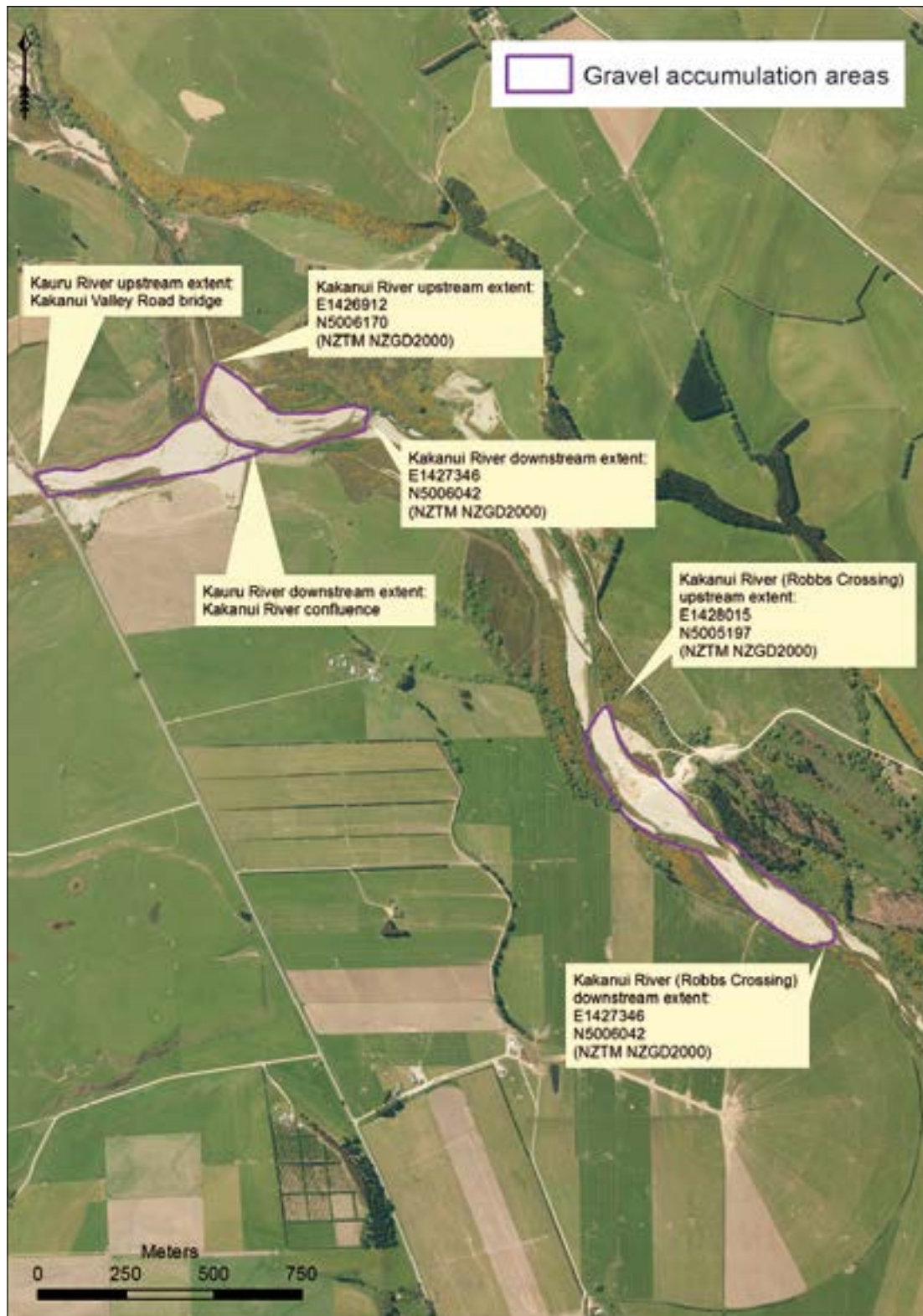
Figure 24. Areas where gravel tends to naturally accumulate in the Kākaunui and Kauru rivers; near the Kākaunui / Kauru confluence, and at Robbs Crossing (outlined in pink). The upstream and downstream extents are also identified.
