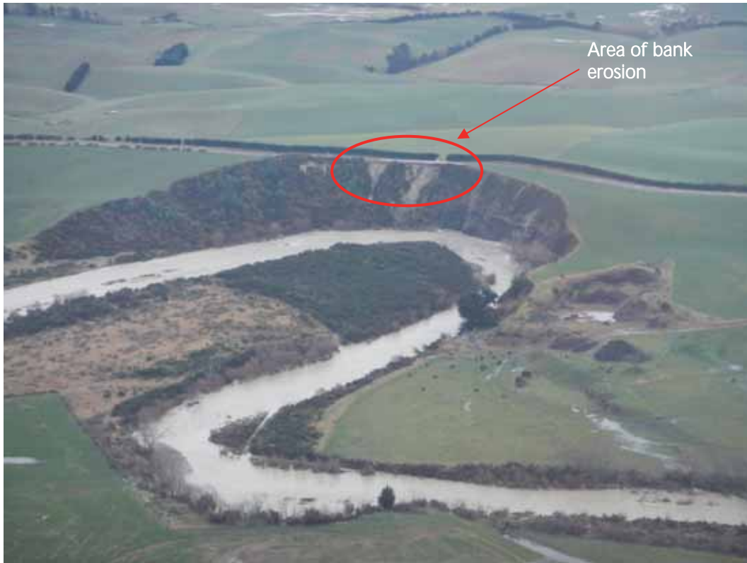
Figure 7 Aerial view of the Waianakarua River looking upstream during a period of high flow in August 2012. The location of Figure 6 is circled in red.
