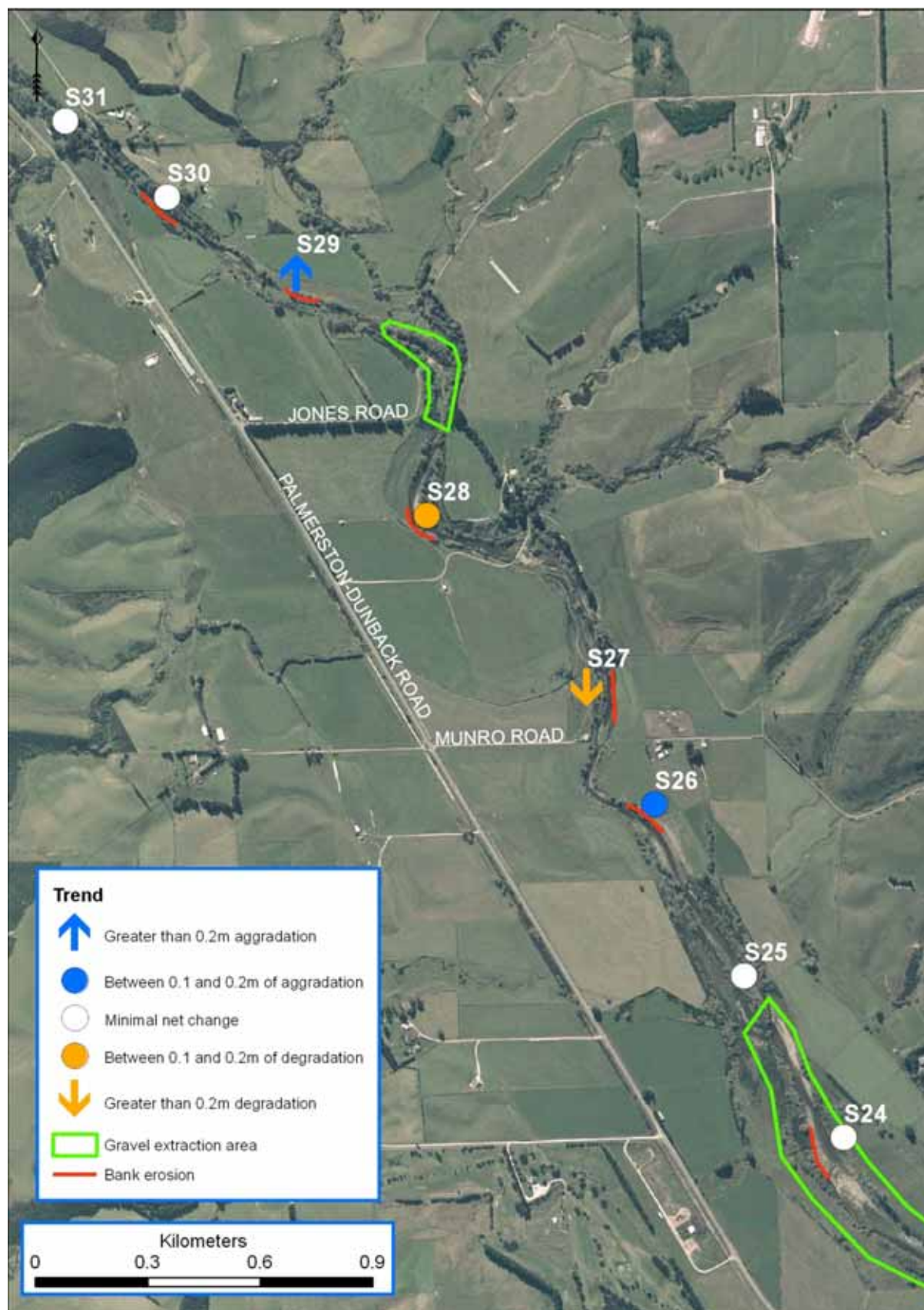
Figure 8. The location of cross-sections S31 to S24 on the Shag/Waihemo River. The white, orange, and blue symbols show the magnitude of MBL change at each cross-section between April 2009 and October 2013. Locations where significant bank erosion (>1m) was observed during this period are shown as red lines. Locations of historic gravel extraction are outlined in green.
