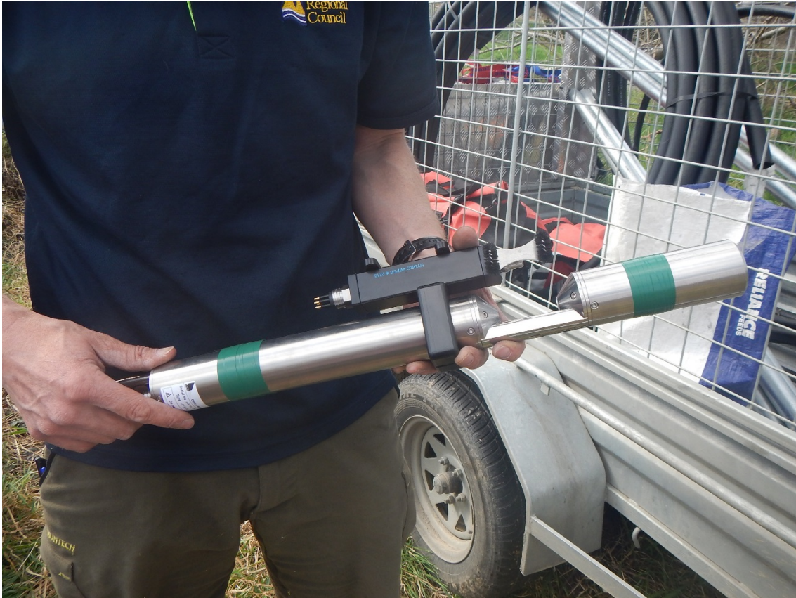
Figure 4. The TRlos continuous nitrate sensor with a wiper system designed to eliminate fouling of the lenses.
