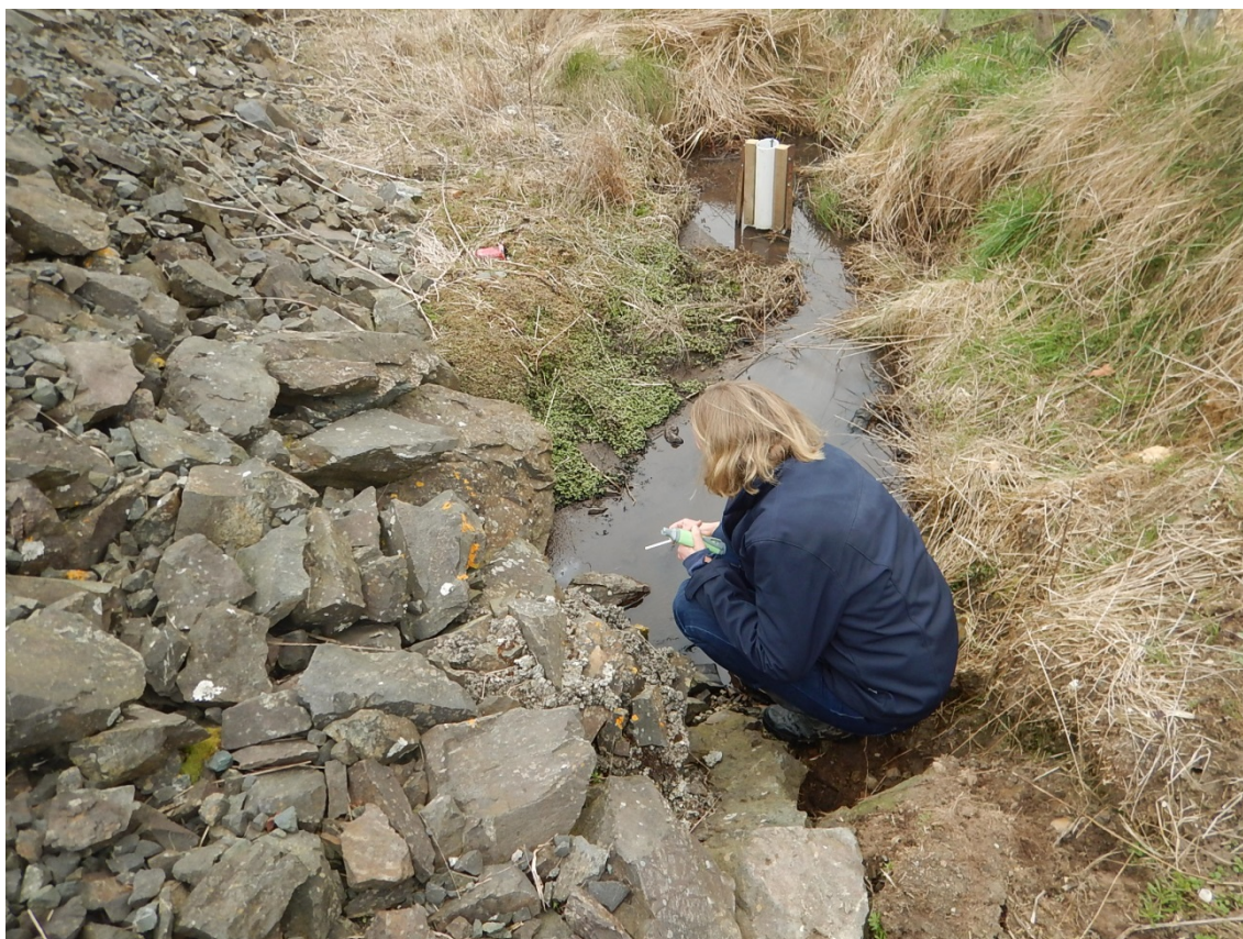
Figure 1. Rachel Ozanne (water quality scientist) takes a grab sample next to the conductivity monitor set up by AgHub.
