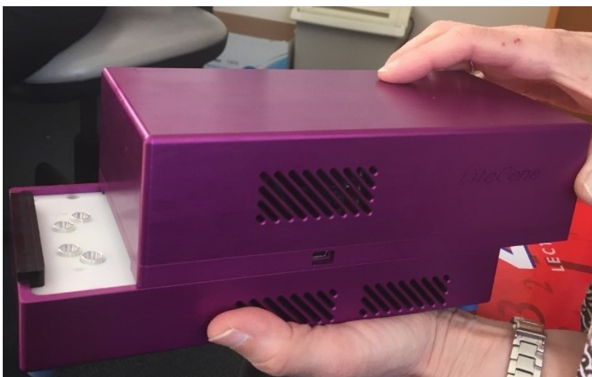
Figure 2. The Freedom4 component of a system designed to rapidly detect and quantify microbials. Four sampling ports can be seen on the lefthand side.
