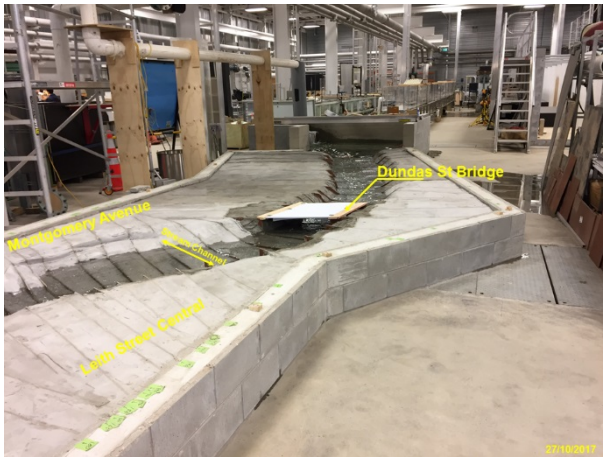
Figure 4. Calibration of the physical model of the Water of Leith near Dundas Street at the University of Auckland. The photograph is looking upstream.
