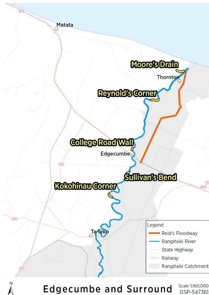
Figure 33: Edgcumbe area and critical structures related to the 2017 flood event (Source: Bay of Plenty Regional Council 2017)
