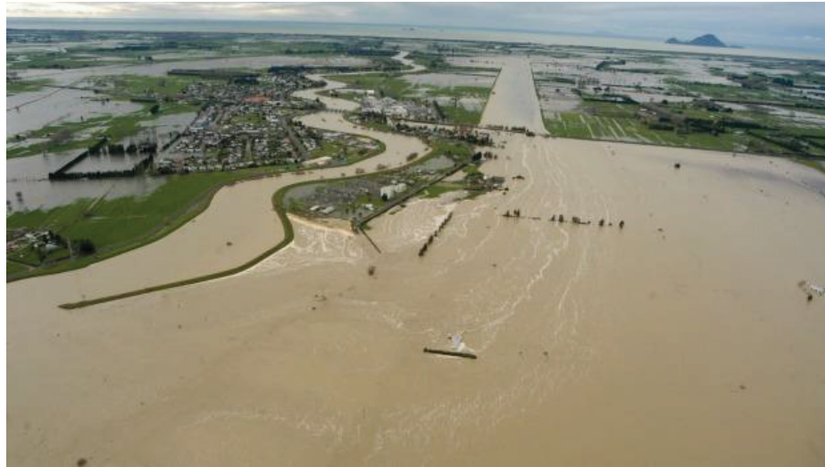
Figure 27: 2004 Flood showing effects of breach and overflows into Reid's Floodway (Source: Whakatāne Beacon)
