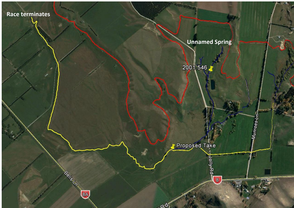
Figure 2. Map showing the Unnamed Spring (in blue) and the existing take from it (2001.546) as well as the “proposed take”. Also shown is the LIC main race (in red) and the Lower LIC race (in yellow) including where the race terminates.
