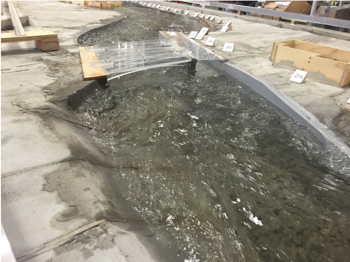
Figure 11: Physical modelling of new culvert at Dundas Street bridge at a flow of 171 m 3 /s (model scale 1:25). The photograph is looking downstream with the culvert at the true right side of the channel.
