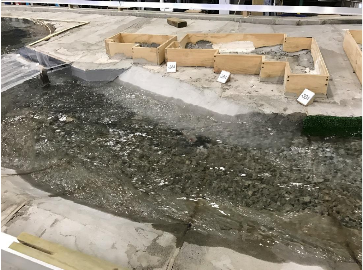
Figure 4: The proposed Dundas Street culvert and upstream retaining wall at an equivalent design flow of 171m 3 /s (100-year Return Period). The flow is from right to left. The existing Dundas Street bridge and proposed new culvert are at the top left of photograph. The wooden objects are buildings.
