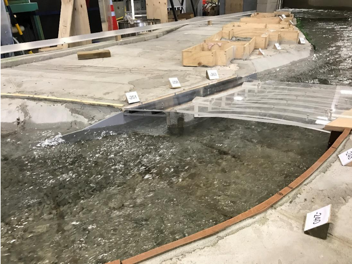
Figure 5: The proposed Dundas Street culvert and downstream retaining wall at an equivalent flow of 140^3\text{m}^3/\text{s} . The photograph is looking upstream. The proposed new culvert is at the centre of the photograph.
