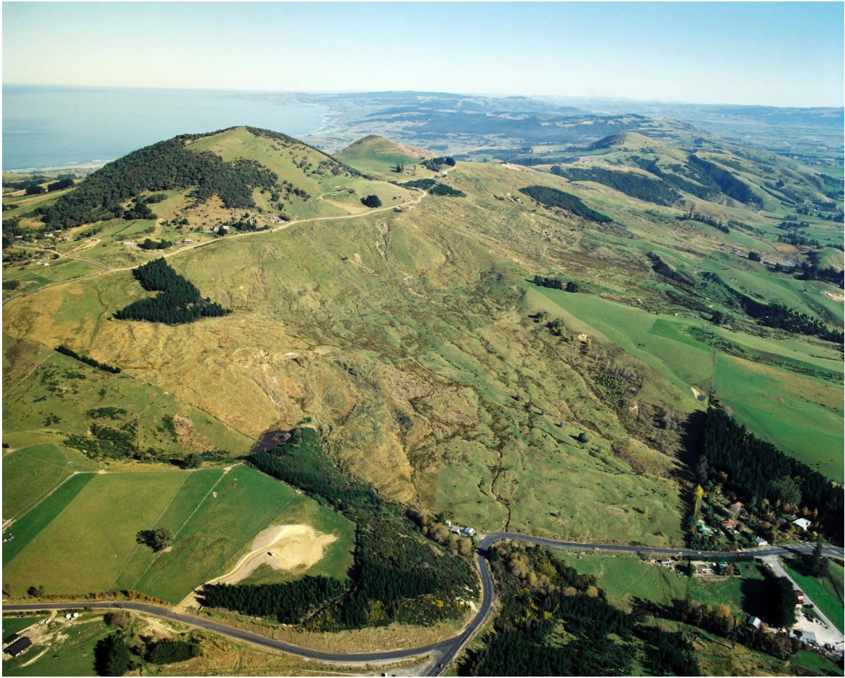
Figure 6.2 Evidence of historic landslides on the northern flanks of Saddle Hill. The cap of the hill is covered in resistant Dunedin volcanic rock, underlain by Henley Breccia. Source: GNS Science
