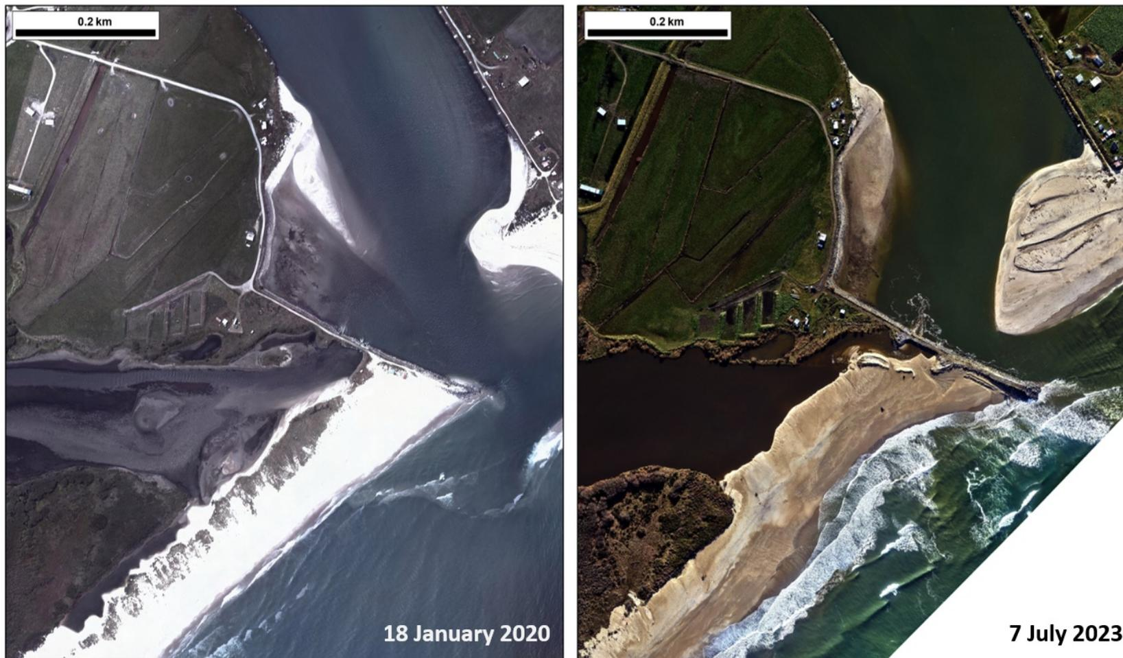
Figure 3: Aerial imagery showing the Koau Mouth of the Clutha River / Mata-Au in January 2020 (left), and July 2023 following the coastal erosion event (right).
