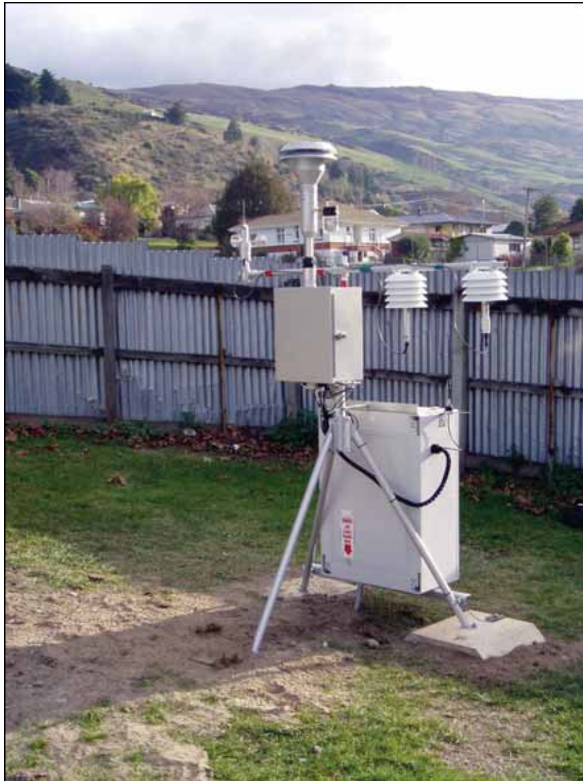
Figure 2.6 A typical continuous beta monitoring site
