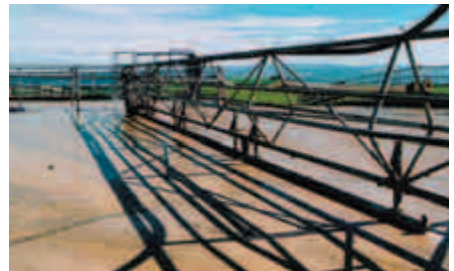
Dungbuster used to reduce the amount of washdown water.
