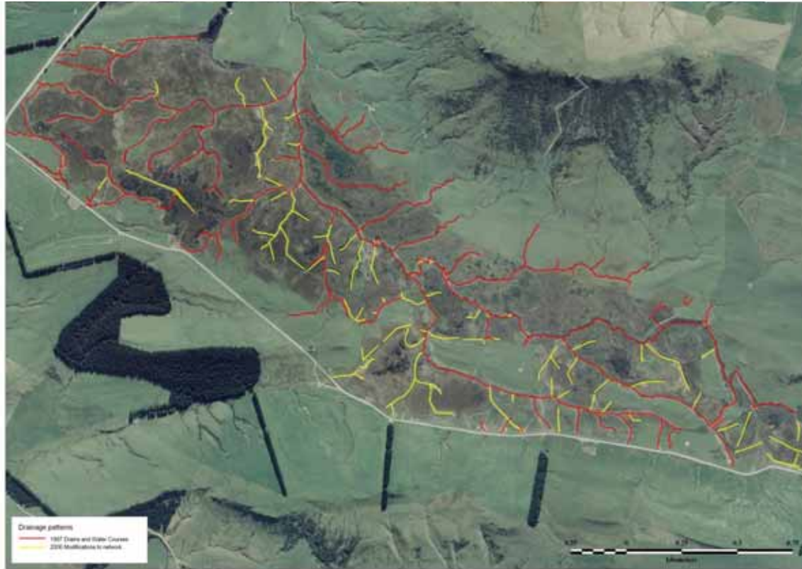
Figure 5-4 Cairn Swamp Wetland showing the increased drainage network comparing 1997 (red line) to 2006 (yellow line)
