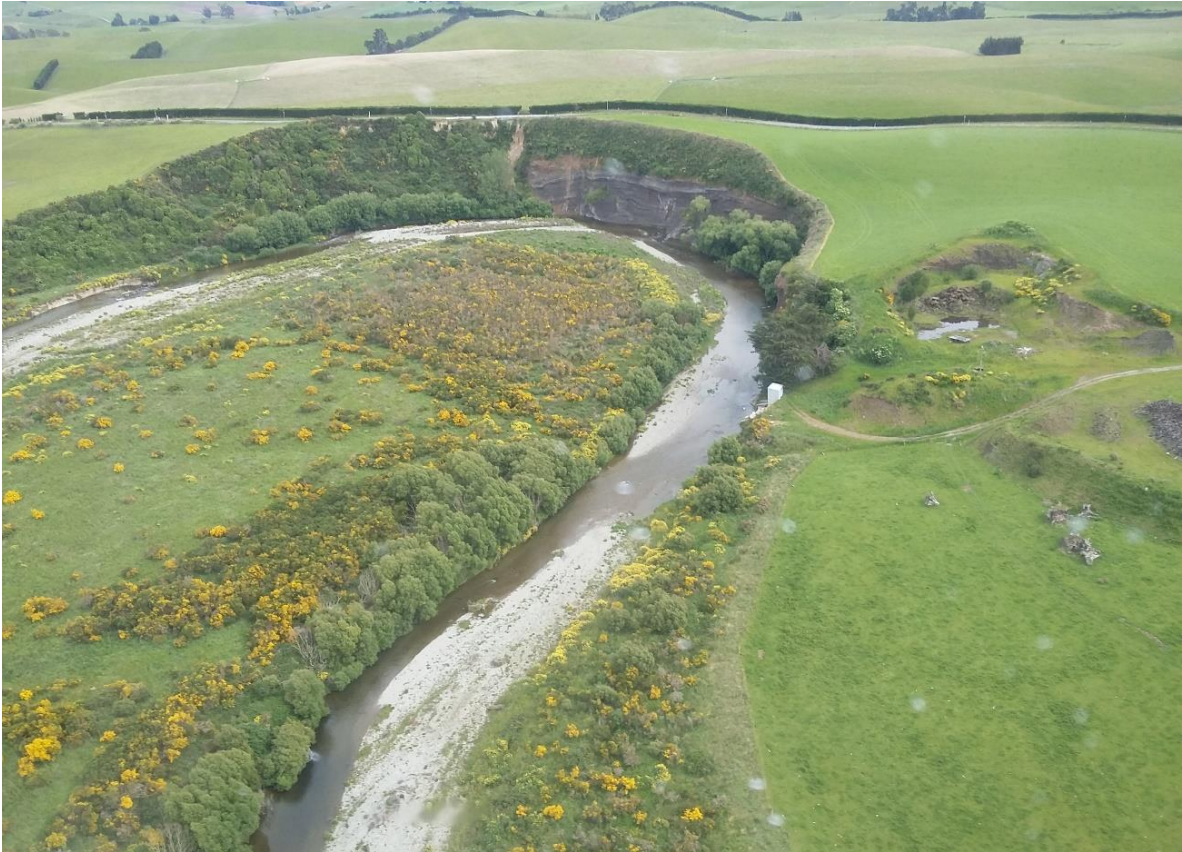
Figure 3. Examples of changes in channel morphology. Top: Bank erosion on the true-left bank of the Waianakarua River (Summer 2014/15). Bottom: Bank erosion at a bend of the Waianakarua River adjacent to Waianakarua Road. The establishment of invasive weed species on the inner bend of the channel, reduces the lateral confines of the channel.
