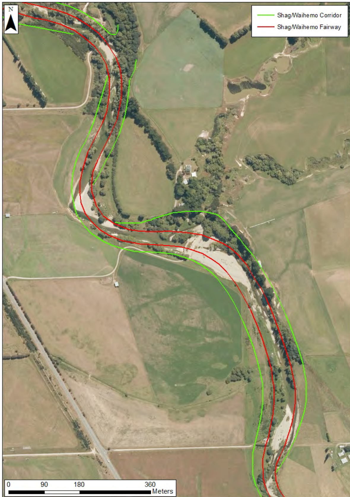
Figure 18. Shag River/Waihemo River mapped fairway deviating from the current channel alignment (aerial photography collected in 2014)
