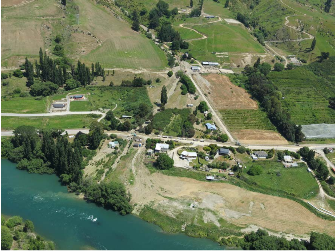
Figure 3.16 The Pump Station Creek debris flow fan showing the two avulsion sites, one near the fan-head and the other at SH8 (Photo: Ben Mackey, ORC; 27/11/2017).
