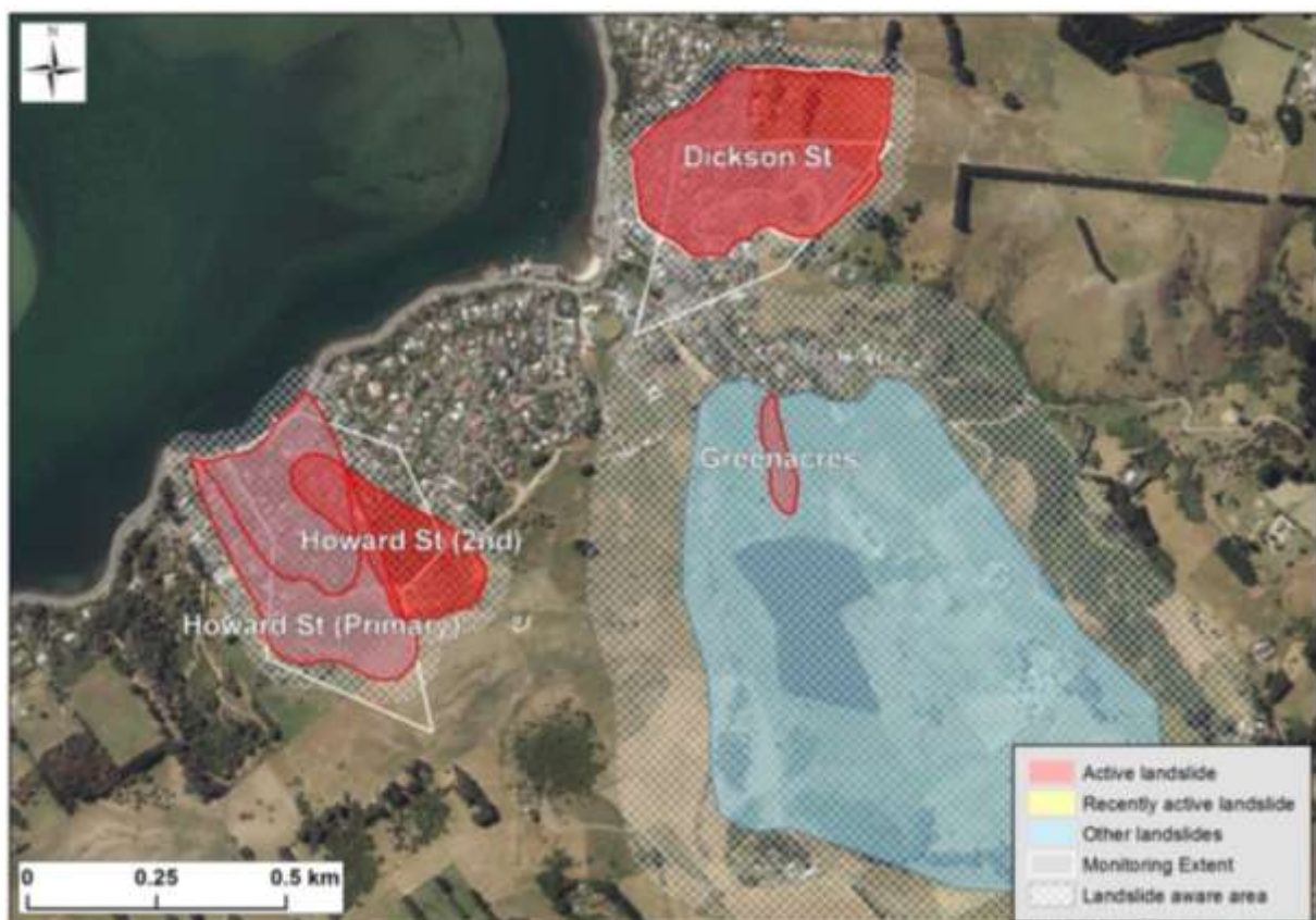
Figure 10 An active earthflow within the larger Greenacres Mass Movement Area (shaded blue). Signs of activity on the earthflow were observed in June 2015.
