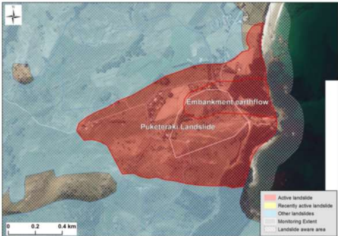
Figure 18 The Puketeraki landslide and Embankment earthflow. These active landslides are surrounded by landslides currently assessed as inactive.
