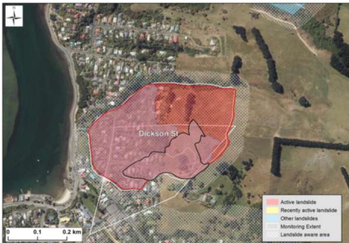
Figure 9 The Dickson Street Slide. The internal area of the slide (black outline) was assessed by Barrell et al., 1994. The larger red outline is from Johnson, 1987.
