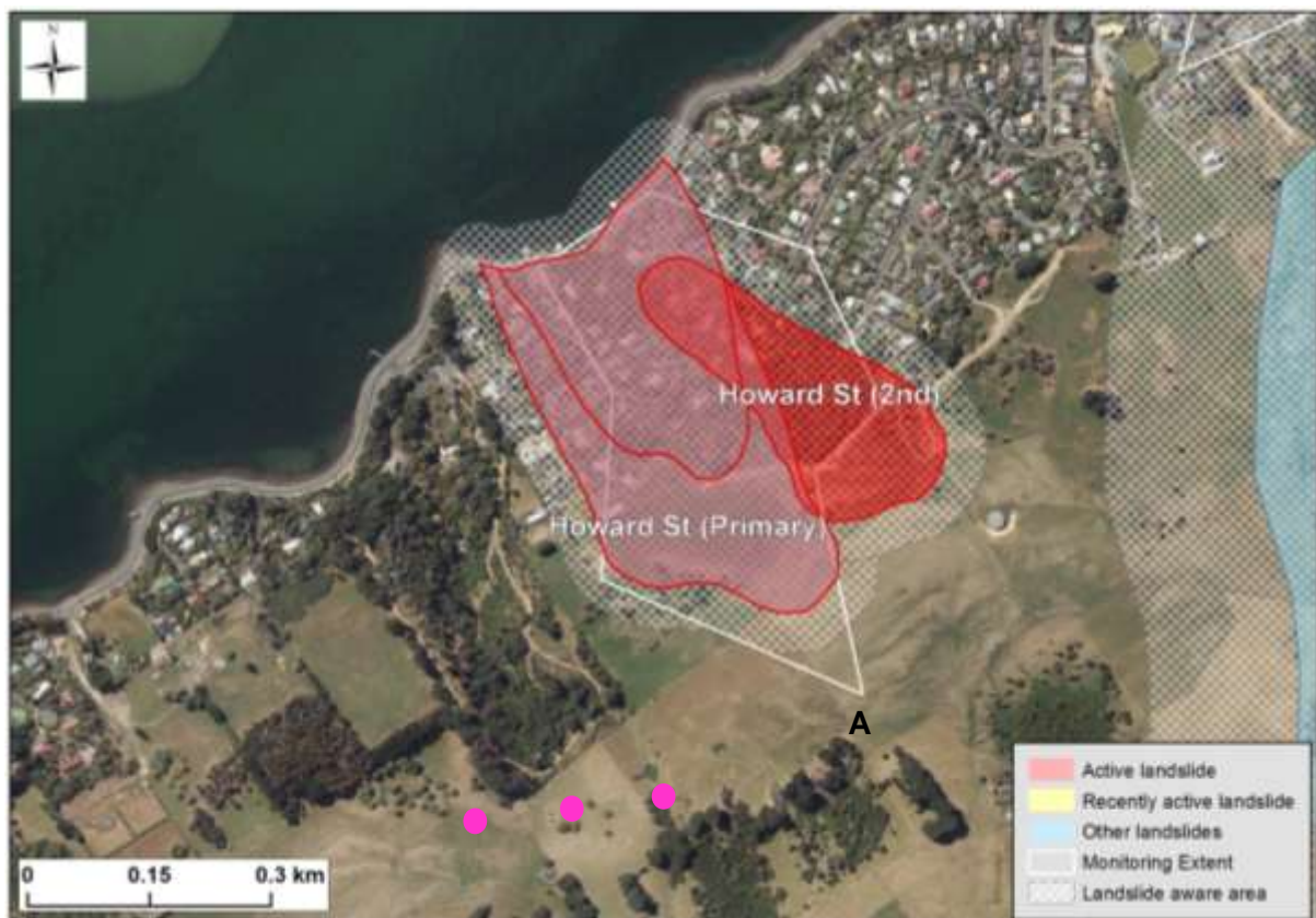
Figure 12 Howard Street landslides. The approximate location of surficial landslides observed in June 2015 are shown (pink circles), and the uppermost survey point is labelled 'A'.
