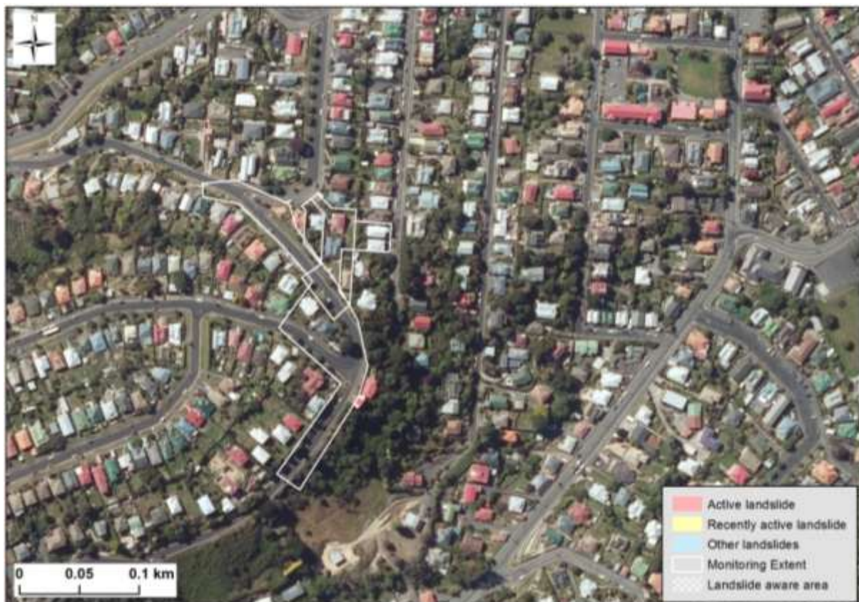
Figure 27 Sidey Street Slide area, showing the extent of the monitoring conducted by the DCC
