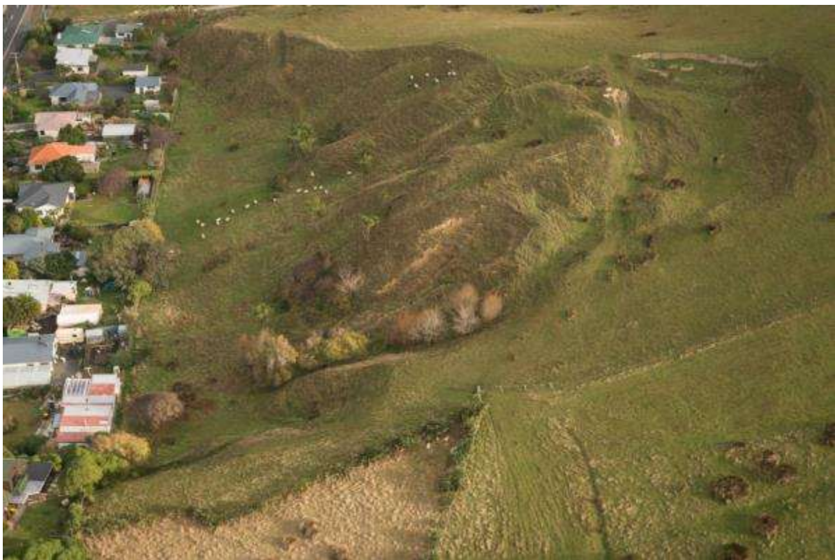
Figure 5 Brighton Slide from the air, looking towards the west, 16 June 2015. The landslide mass in the center of the image is the active part of the slide.
