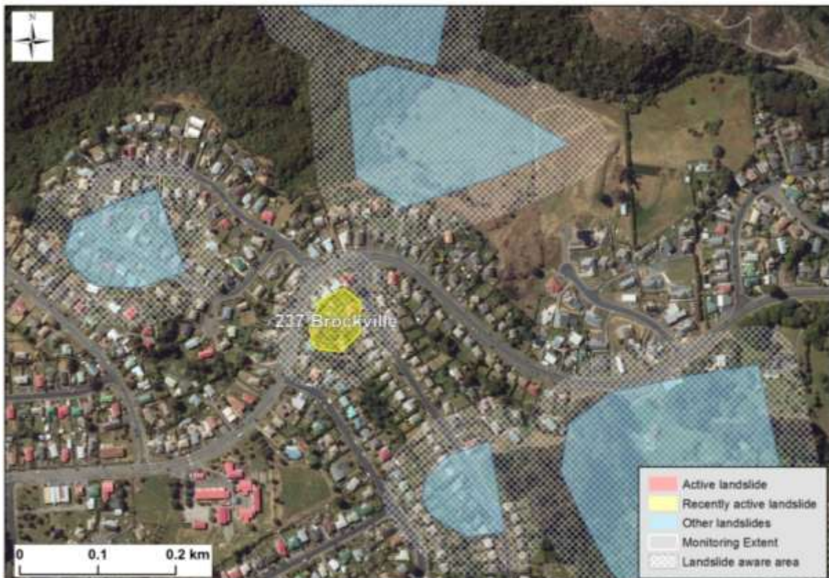
Figure 22 237 Brockville Road Landslide
