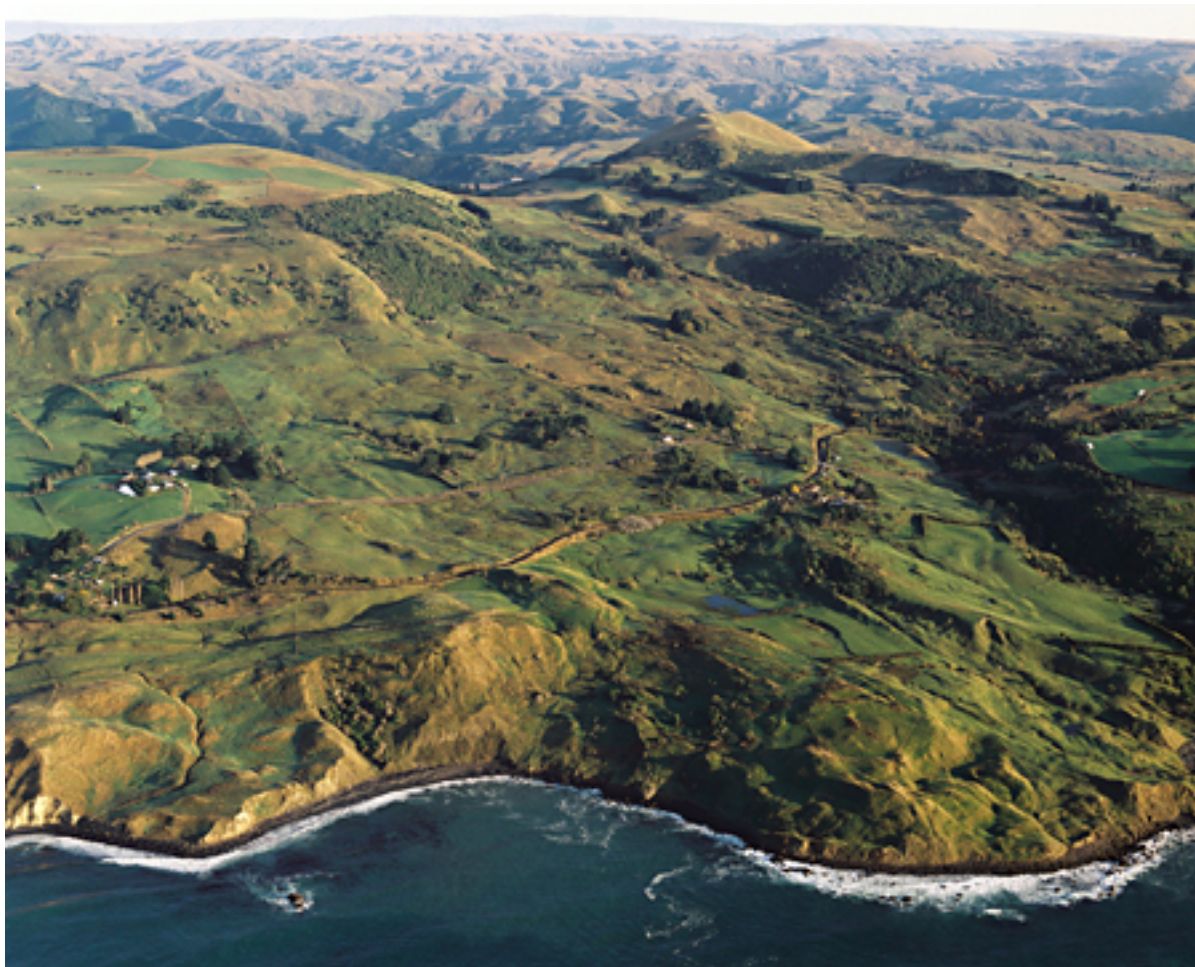
Figure 13 Typical earthflow ‘hummocky’ terrain Warrington to Karitane. Most of the land between the coast and the flat topped ridge is landslide. The Scenic Coast Road and the South Island Main Trunk railway cross the centre of photo (GNS Science, CN26986-03, Photographer, L. Homer).
