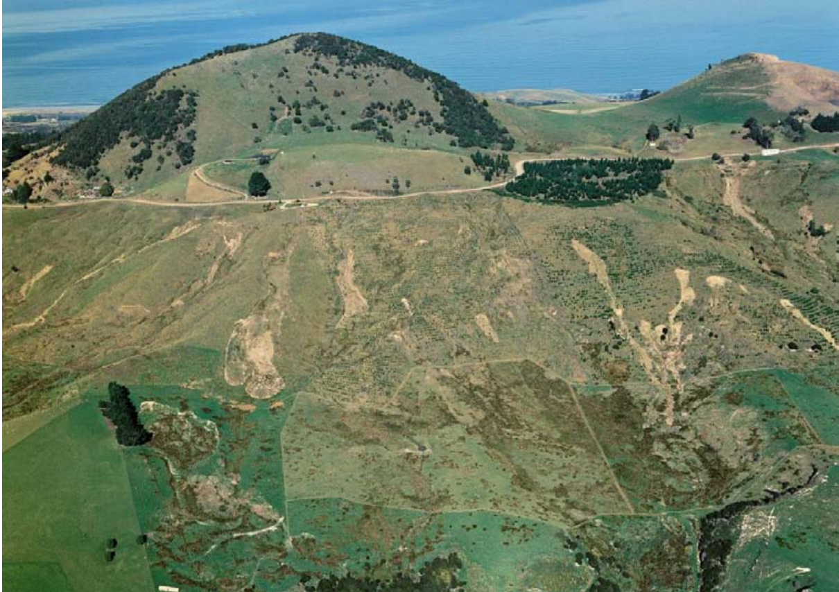
Figure 7 An aerial view south towards Saddle Hill Road, running left-right, above which rise the promontories of Saddle Hill (left) and Jaffray Hill (far right). From Saddle Hill Road to below the bottom of the photo is a moderate slope descending towards the Taieri Plain (out of sight below the photographer). Much of the slope below Saddle Hill Road is interpreted as a large, deep-seated, bedrock landslide. Superimposed on that landslide are numerous surficial landslides, the freshest of which moved during the March 1994 rainstorm, but many older, more subdued, scars relate to previous recent historical activity. This area is clearly very susceptible to landsliding. The young trees evident in this photo are now mature, and today obscure much of the detail of past landsliding on this slope. Photo: GNS Science CN 32285b, D.L. Homer, 1 May 1994,
