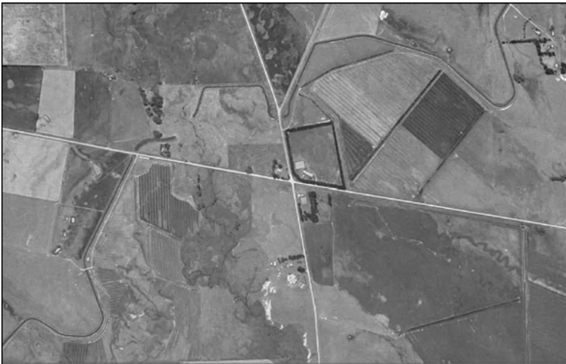
Figure 5.8 Aerial photograph of flood irrigation and drainage channels in area bounded by rectangle in Figure 5.7. The MIC scheme can clearly be seen as it passes under the Wether Burn
