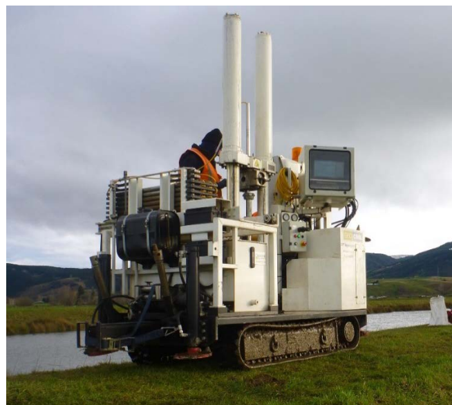
Figure 7: A cone penetrometer (CPT) rig testing ORC's floodbanks on the Taieri Plain in 2015.
