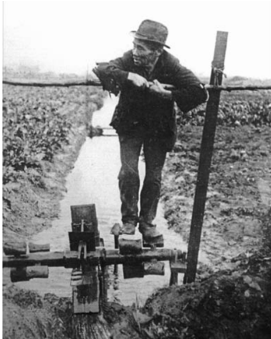
Figure 3: Market gardener operating a land drainage pump in South Dunedin in the late nineteenth century.
