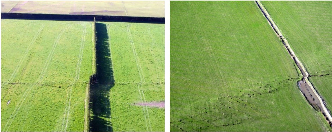
Figure 5.2 Example of surface-fault rupture on the Canterbury Plains after the Mw 7.1 Darfield earthquake, in September 2010. An average horizontal displacement of 2.5m was recorded along this fault (Quigley, et al. , 2011). (Photograph source, GNS Science).
