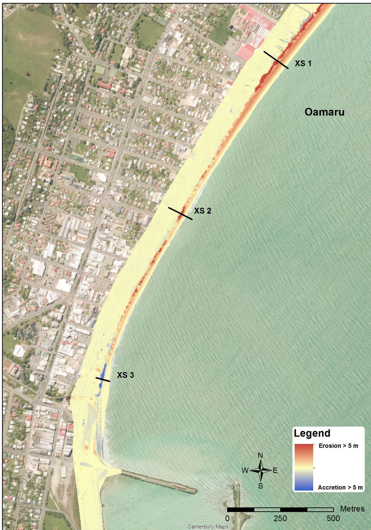
Figure 3-24: Difference in elevation between 2004 and 2016 near Oamaru based on LiDAR surveys.
