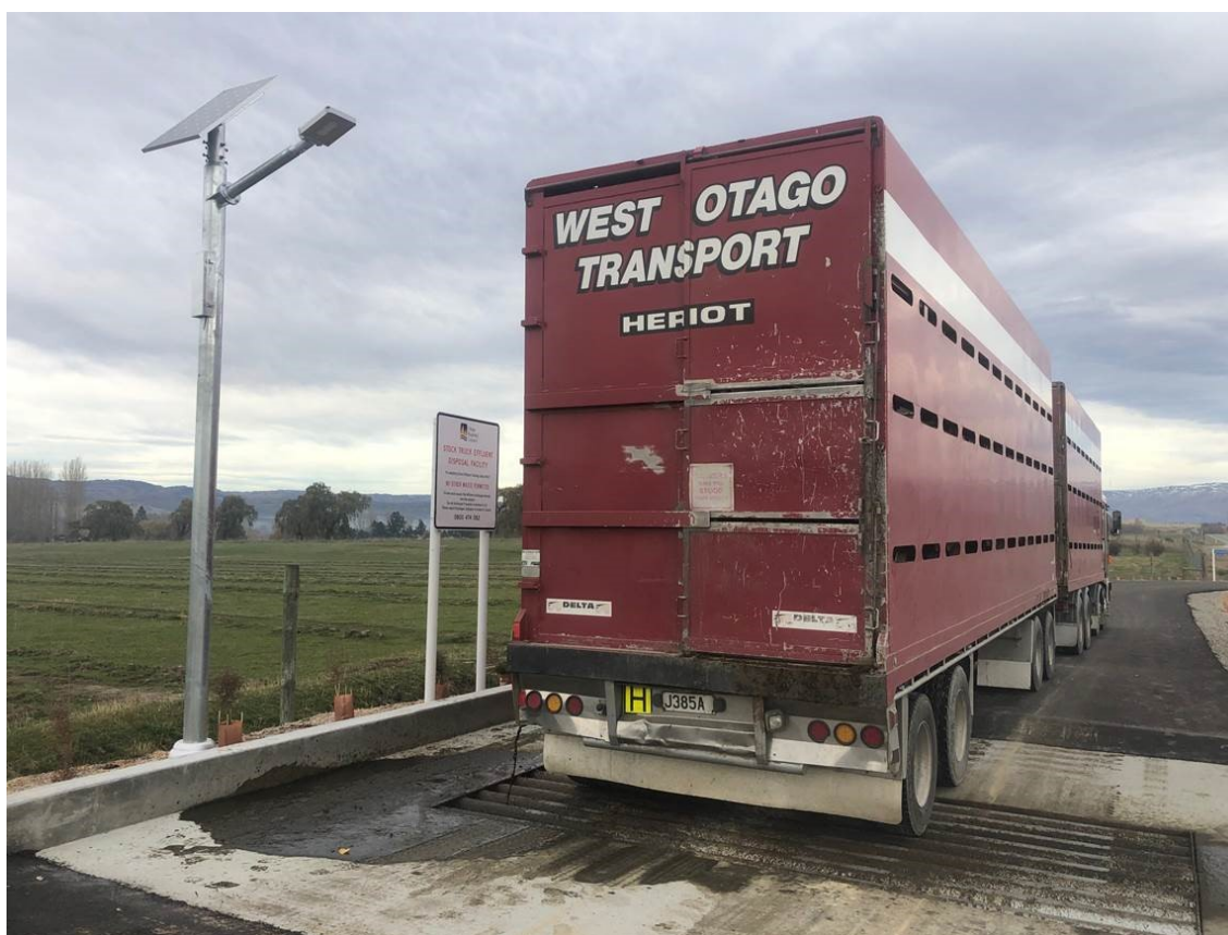
Figure 11: Stock truck discharging effluent into the SH85 (Brassknocker Road) STED on 26 May 2019 (photograph courtesy Bruce Robertson, Road Transport Logistics Ltd, Tapanui)
