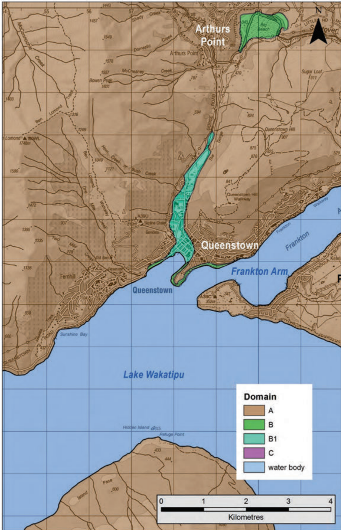
Figure A3.3 Liquefaction-susceptibility domains in the Queenstown area. The key is generic to the dataset and not all units may be present on this map.
