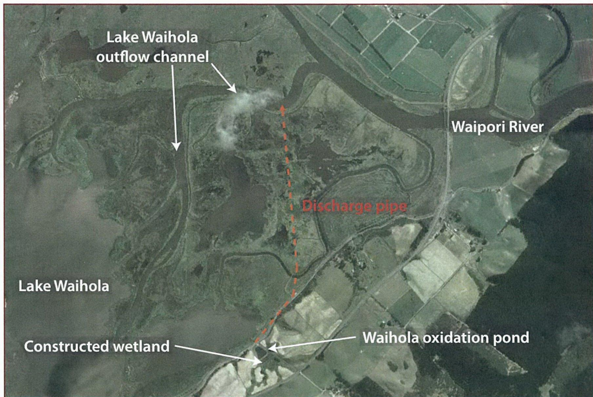
Figure 3 Aerial photograph of the Lake Waihola outflow channel and nearby Waihola oxidation pond, Otago. A dashed red line indicates the approximate path of the oxidation pond discharge pipe (satellite imagery courtesy of Google maps).
