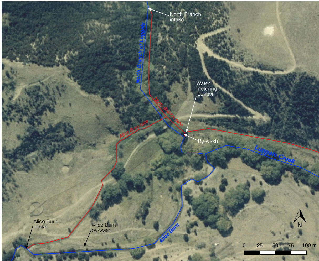
Figure 4 Map of the confluence of Luggate Creek and Alice Burn showing irrigation races and by-washes.
