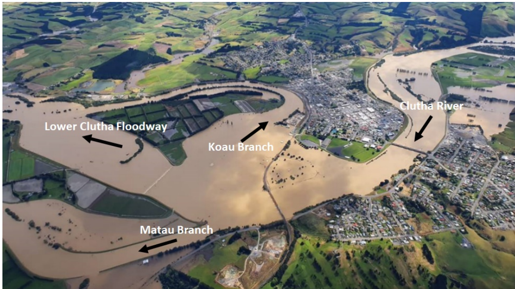
Figure 14. Impact on Lower Clutha Flood Protection and Drainage Scheme in vicinity of Balclutha (5 February 2020, flow in the Clutha River was 3,058m 3 /s approximately (the river peaked at 3,179m 3 /s on 5 February 2020 at 10am approximately) (Photo: Landpro)
