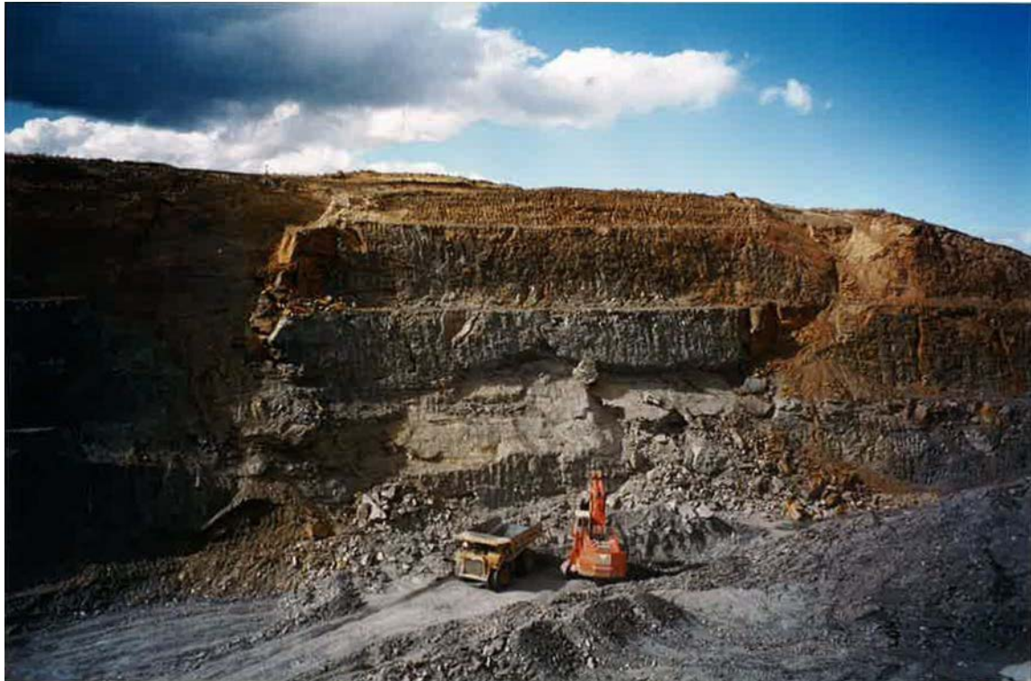
Photograph 2: View of east wall multi bench failure at Deepdell
