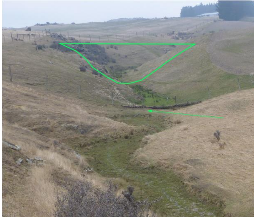
Figure 5: Gully located in a tributary of Highlay Creek, August 2019. Green outline indicates general area where a haul road and culvert are to be located. Arrow shows the raised bank that the deer fence sits on.
