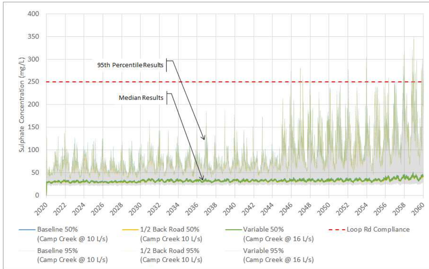
Figure 10: Predicted Sulphate concentrations over time at Shag River (50th and 95th percentile values)
