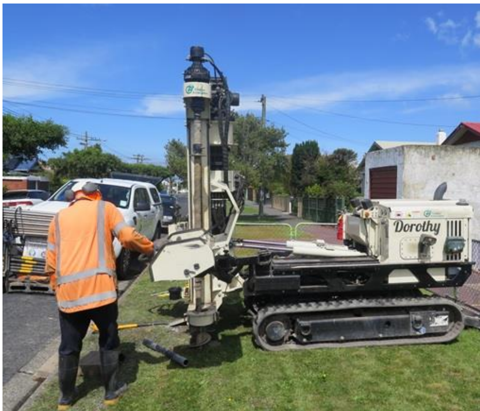
Figure 1. Cone Penetrometer Testing (CPT) rig taking pressure readings from the soil beneath South Dunedin in 2019.
