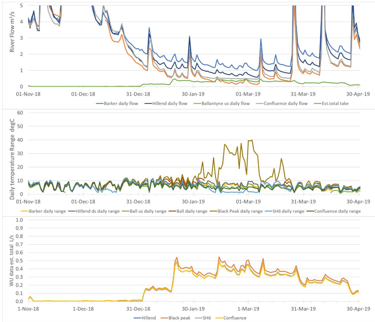
Figure 7-6: Flows, temperature ranges and estimated water use in the lower Cardrona River, 1 November 2018 to 1 May 2019. The top plot shows flow and water use in cumecs; the middle plot shows temperature range in degrees C, and the lower plot shows an expanded view of the estimated water use in cumecs.
