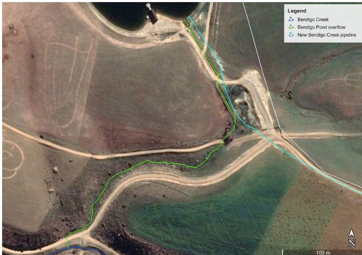
Figure 7: Bendigo Pond overflow path and discharge back to Bendigo Creek
