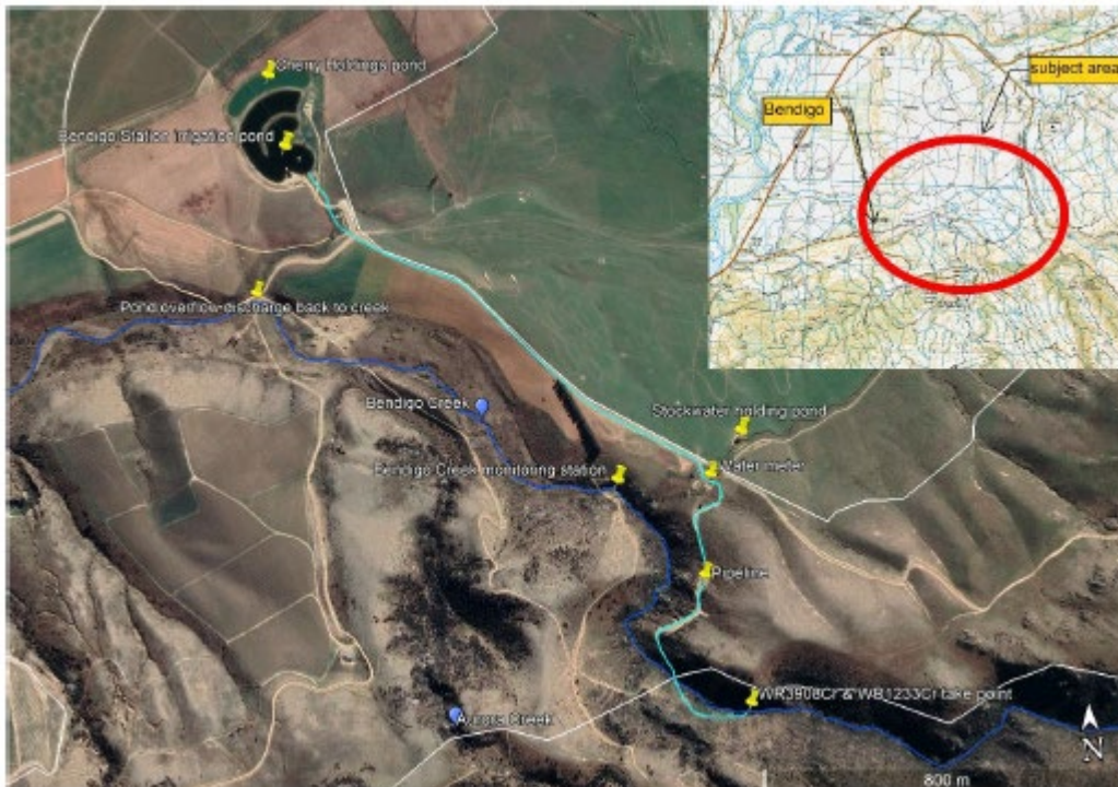
Figure 1: Annotated aerial photograph showing point of take, water conveyance and reservoirs. Source: Application.
